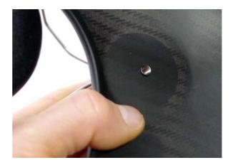
Place the steel washer onto the hollow bolt, and then insert the hex drive screw.
