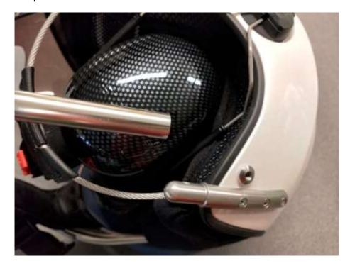
• Fasten the rollbar using the two crosshead screws, screwing them into the hole on the inside of the rollbar near where it is attached to the helmet.
