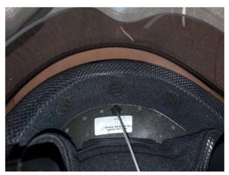
• While looking into the hole, move the visor until the screw comes into view (you will see it when the visor is about two-thirds fully down).
