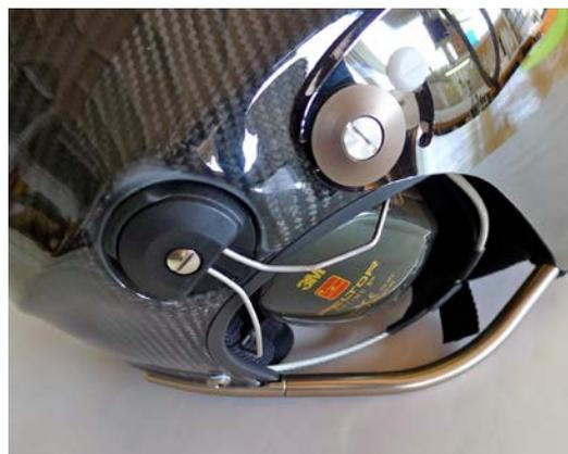
To install the earphones, the polystyrene inner lining has to be removed.
