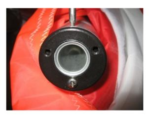
Using a pair of needle-nose pliers pushed into the two holes in the head of the cam, rotate the cam
