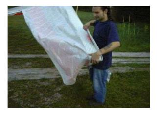
• Holding the extremity of the wing in this position, take the sail by the trailing edge and lift it upwards until it is tight and from this position roll in the sail, starting from the trailing edge.
