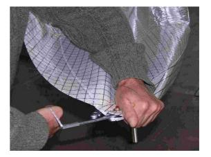
Using the attached cord, push the tip-lever into the sail until it "clicks" against the fibreglass tip. The sail is now tensioned.
